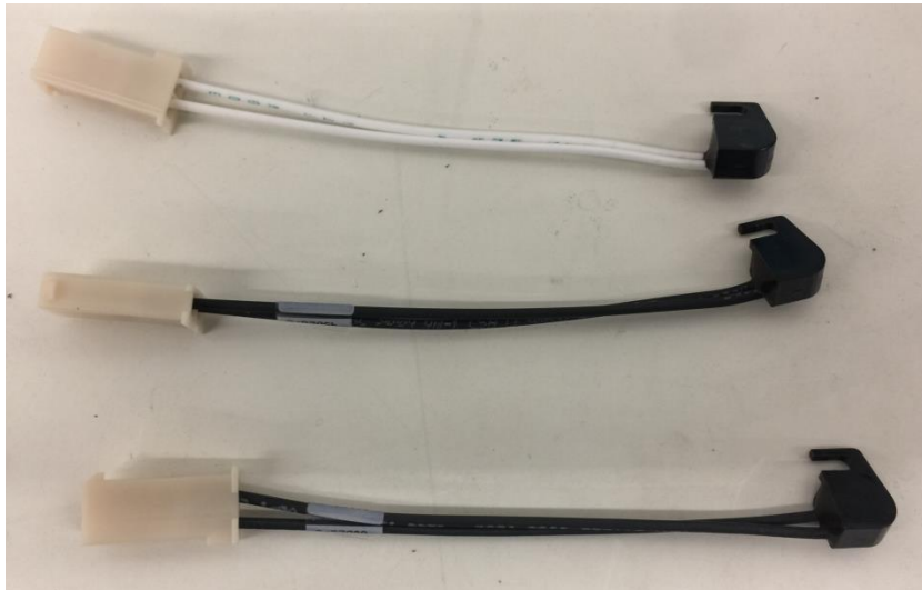
Snap switches: 160°C, 95°C, 65°C (top to bottom, labeled)
