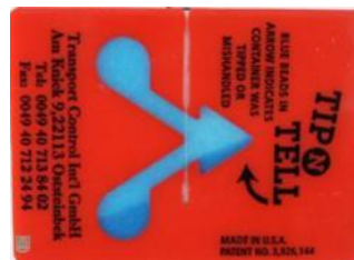
TIP N TELL – Bad Shipment with Failed (Blue) Indicator
